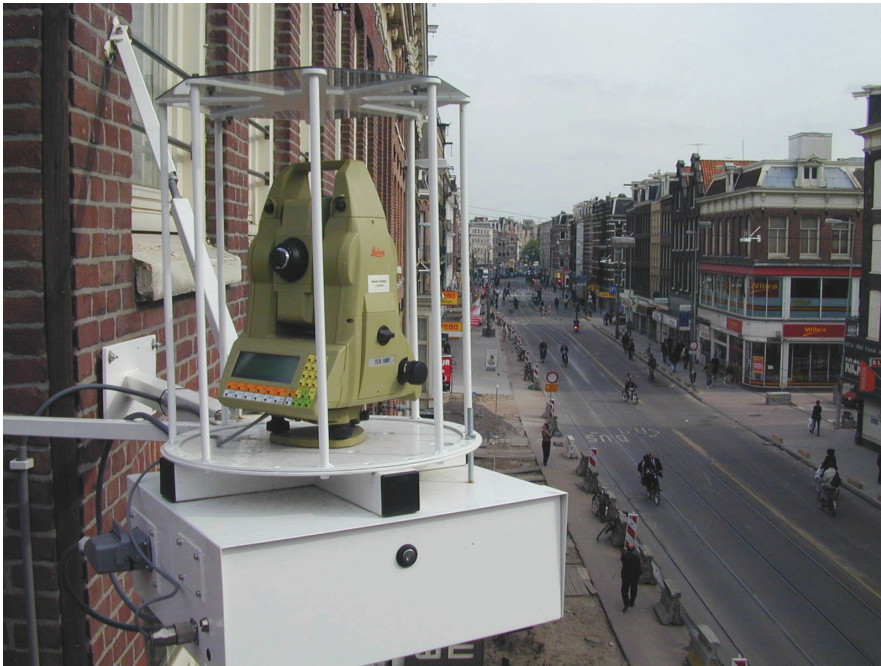
Figure 1. Typical RTS installation – (Photograph courtesy of SolData; all rights reserved).
